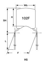
Component outline for lead spacing 5.0 mm  $\pm$  0.8 mm (flat bent leads)
