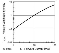
Fig. 6 - Relative Luminous Intensity vs. Forward Current
