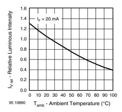
Fig. 4 - Relative Luminous Intensity vs. Ambient Temperature
