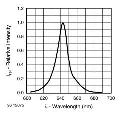
Fig. 7 - Relative Intensity vs. Wavelength
