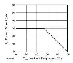
Figure 2. Forward Current vs. Ambient Temperature for InGaN
