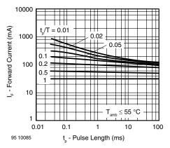
Figure 3. Forward Current vs. Pulse Length
