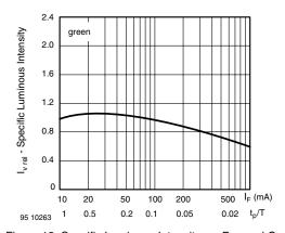
Figure 12. Specific Luminous Intensity vs. Forward Current
