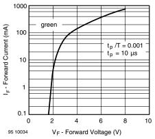
Figure 10. Forward Current vs. Forward Voltage
