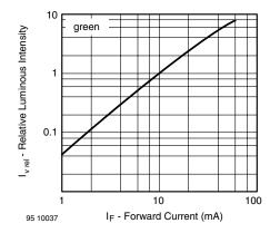
Figure 13. Relative Luminous Intensity vs. Forward Current
