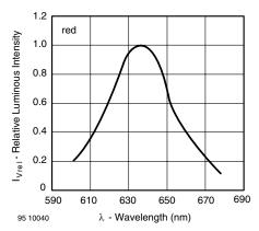
Figure 9. Relative Intensity vs. Wavelength
