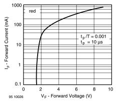
Figure 5. Forward Current vs. Forward Voltage
