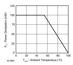
Figure 1. Power Dissipation vs. Ambient Temperature
