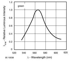
Figure 14. Relative Intensity vs. Wavelength
