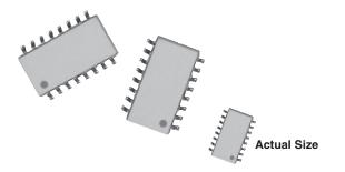
Vishay Dale Thin Film offers standard circuits in 16 pins in a medium body molded surface mount package. The networks are available over a resistance range of 100  $\Omega$  to 100 k $\Omega$ . The network features tight ratio tolerances and close TCR tracking. In addition to the standards shown, custom circuits are available upon request.
