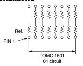
The 01 circuit provides 15 nominally equal resistors, each connected between a common lead (16) and a discrete PC board pin.
