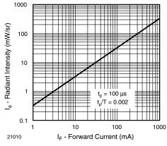
Fig. 4 - Radiant Intensity vs. Forward Current
