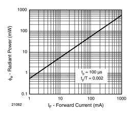
Fig. 5 - Radiant Power vs. Forward Current
