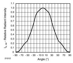
Fig. 7 - Relative Radiant Intensity vs. Angular Displacement
