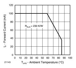
Fig. 1 - Forward Current Limit vs. Ambient Temperature
