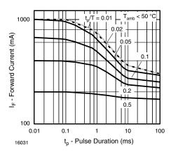
Fig. 2 - Pulse Forward Current vs. Pulse Duration
