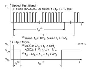
Fig. 1 - Output Delay and Pulse-Width
