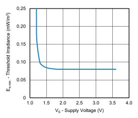
Fig. 12 - Sensitivity vs. Supply Voltage
