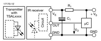
$R_1$  and  $C_1$  recommended to reduce supply ripple for  $V_S < 2.2 \text{ V}$
