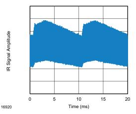
Fig. 13 - IR Emission from Fluorescent Lamp With Low Modulation
