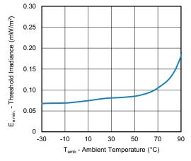
Fig. 9 - Sensitivity vs. Ambient Temperature
