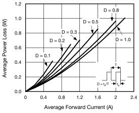
Fig. 2 - Average Power Loss Characteristics
