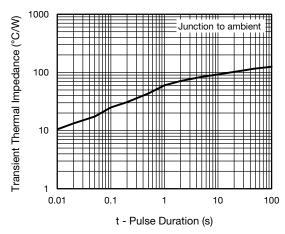
Fig. 6 - Typical Transient Thermal Impedance
