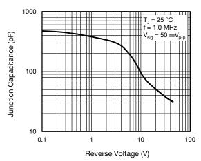
Fig. 5 - Typical Junction Capacitance
