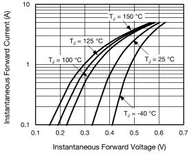
Fig. 3 - Typical Instantaneous Forward Characteristics
