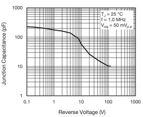
Fig. 5 - Typical Junction Capacitance
