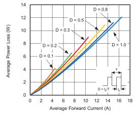
Fig. 2 - Forward Power Loss Characteristics
