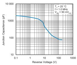
Fig. 5 - Typical Junction Capacitance
