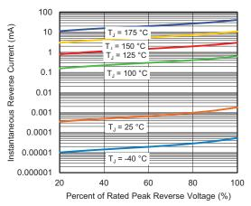
Fig. 4 - Typical Reverse Characteristics
