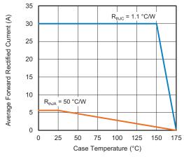
Fig. 1 - Forward Current Derating Curve
