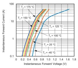
Fig. 3 - Typical Instantaneous Forward Characteristics
