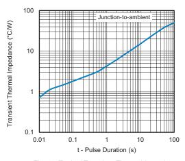
Fig. 6 - Typical Transient Thermal Impedance
