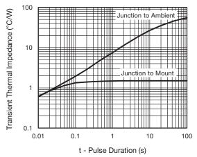
Fig. 6 - Typical Transient Thermal Impedance
