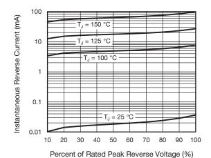
Fig. 4 - Typical Reverse Leakage Characteristics
