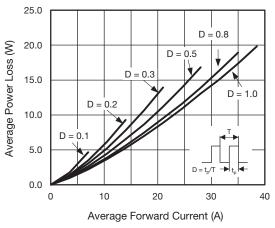
Fig. 2 - Forward Power Loss Characteristics
