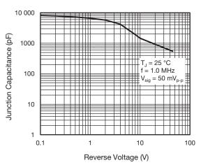
Fig. 5 - Typical Junction Capacitance
