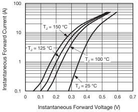
Fig. 3 - Typical Instantaneous Forward Characteristics
