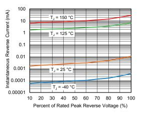
Fig. 4 - Typical Reverse Characteristics
