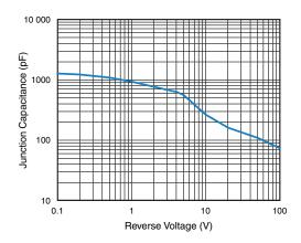
Fig. 5 - Typical Junction Capacitance
