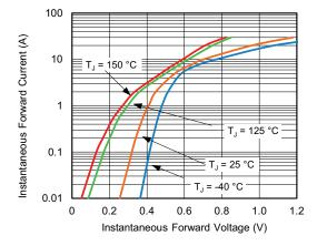
Fig. 3 - Typical Instantaneous Forward Characteristics
