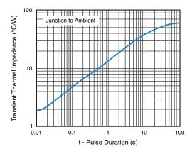
Fig. 6 - Typical Transient Thermal Impedance
