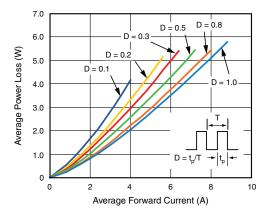
Fig. 2 - Forward Power Loss Characteristics
