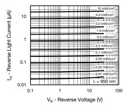
Fig. 4 - Reverse Light Current vs. Reverse Voltage
