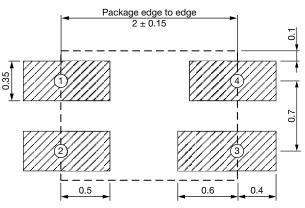
Fig. 9 - VEML3328A3OG PCB Layout Footprint
