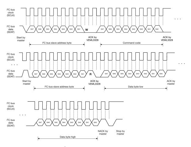
Fig. 3 - I<sup>2</sup>C Bus Timing for Receiving Word Command Format
