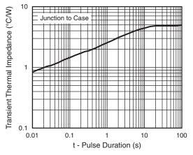
Fig. 5 - Typical Transient Thermal Impedance
