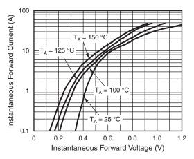
Fig. 3 - Typical Instantaneous Forward Characteristics
