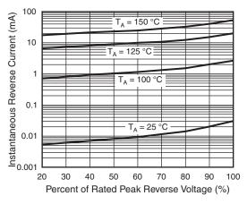
Fig. 4 - Typical Reverse Characteristics
