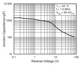
Fig. 6 - Typical Junction Capacitance
