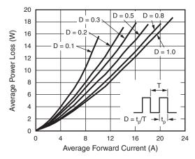
Fig. 2 - Forward Power Dissipation Characteristics
