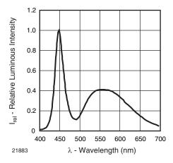
Fig. 4 - Relative Intensity vs. Wavelength
