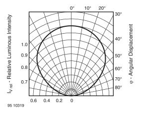
Fig. 5 - Relative Luminous Intensity vs. Angular Displacement
