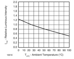
Fig. 7 - Relative Luminous Intensity vs. Ambient Temperature
