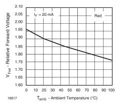
Fig. 8 - Forward Voltage vs. Ambient Temperature
