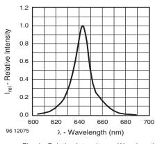
Fig. 4 - Relative Intensity vs. Wavelength
