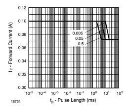
Fig. 2 - Permissible Forward Current vs. Pulse Length
