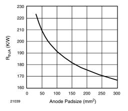
Fig. 5 - Thermal Resistance Junction Ambient vs. Anode Padsize
