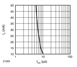
Fig. 9 - Trigger Input Current vs. Turn-on Time
