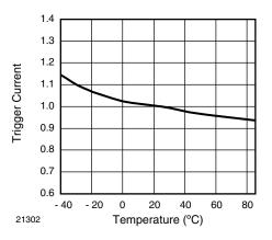
Fig. 8 - Normalized Trigger Input Current vs. Temperature
