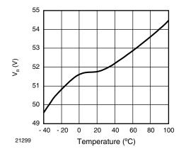
Fig. 5 - Diode Reverse Voltage vs. Temperature
