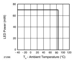
Fig. 1 - Power Dissipation vs. Temperature
