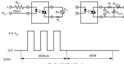
Fig. 3 - dV/dt Test Circuit
