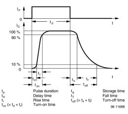
Fig. 5 - Switching Times
