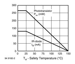
Fig. 1 - Derating Diagram
