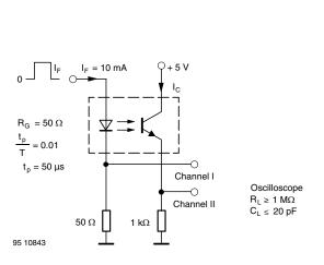
Fig. 4 - Test Circuit, Saturated Operation
