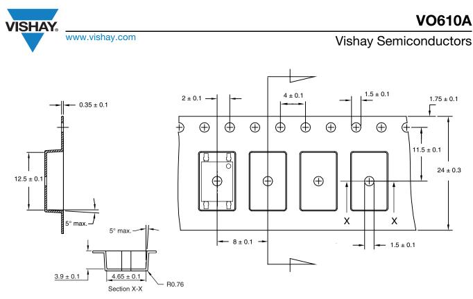
Fig. 8 - Tape and Reel Packing for Option 8 (2000 units per reel)
