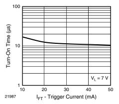
Fig. 7 - Trigger Current vs. Turn-On Time
