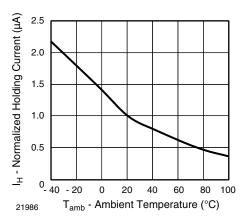
Fig. 8 - Normalized Holding Current vs. Ambient Temperature
