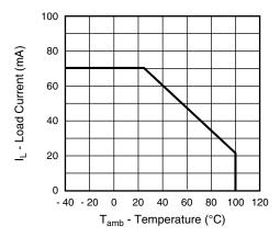
Fig. 1 - Recommended Operating Condition
