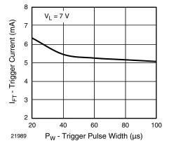
Fig. 10 - Trigger Current vs. Trigger Pulse Width
