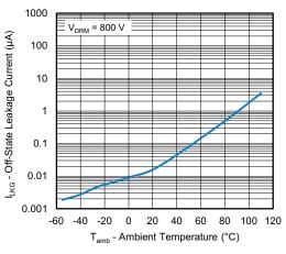
Fig. 8 - Off-State Leakage Current vs. Ambient Temperature
