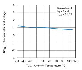
Fig. 11 - Normalized Inhibit Voltage vs. Ambient Temperature
