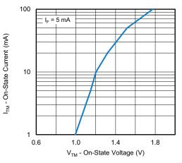
Fig. 6 - On State Current vs. On State Voltage
