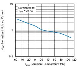
Fig. 7 - Normalized Holding Current vs. Ambient Temperature
