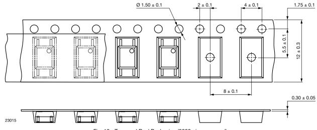
Fig. 13 - Tape and Reel Packaging (3000 pieces on reel)
