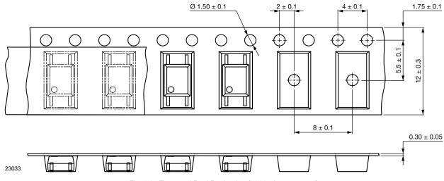
Fig. 14 - Tape and Reel Packaging (3000 pieces on reel)
