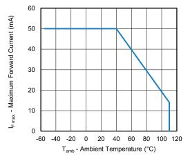
Fig. 1 - Maximum Forward Current vs. Ambient Temperature
