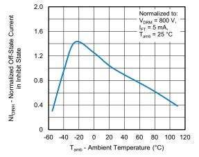
Fig. 9 - Off-State Current in Inhibit State vs. Ambient Temperature
