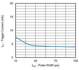
Fig. 5 - Trigger Current vs. Pulse Width
