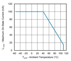
Fig. 2 - Maximum On-State Current vs. Ambient Temperature
