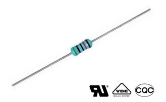
A metal glazed film is deposited on a high grade ceramic body. After a helical groove has been cut in the resistive layer, tinned electrolytic copper wires are welded to the end-caps. The resistors are coated with a light blue lacquer which provides electrical, mechanical, and climatic protection.
