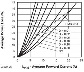
Fig. 6 - Forward Power Loss Characteristics
