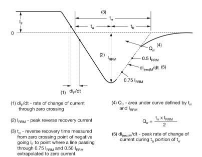
Fig. 9 - Reverse Recovery Waveform and Definitions
