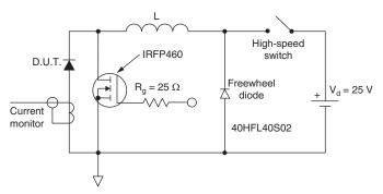
Fig. 8 - Unclamped Inductive Test Circuit
