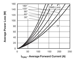
Fig. 6 - Forward Power Loss Characteristics
