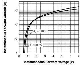
Fig. 5 - Maximum Forward Voltage vs. Forward Current
