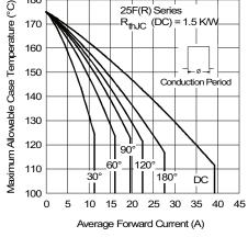
Fig. 2 - Current Ratings Characteristics
