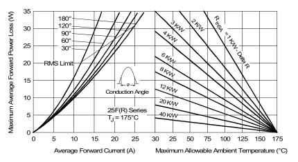
Fig. 3 - Forward Power Loss Characteristics
