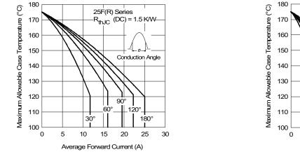
Fig. 1 - Current Ratings Characteristics
