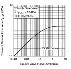
Fig. 8 - Thermal Impedance Z<sub>thJC</sub> Characteristics
