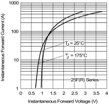
Fig. 7 - Forward Voltage Drop Characteristics
