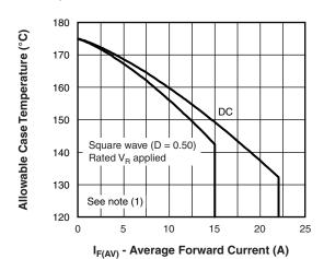
Fig. 5 - Maximum Allowable Case Temperature vs.
