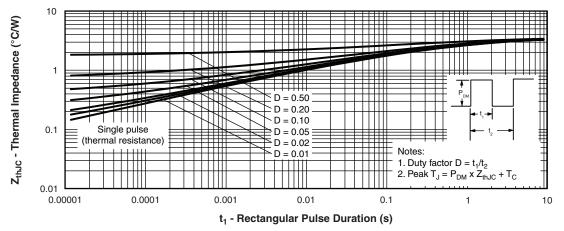
Fig. 5 - Maximum Thermal Impedance ZthJC Characteristics (FULL-PAK)
