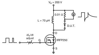
Fig. 11 - Reverse Recovery Parameter Test Circuit
