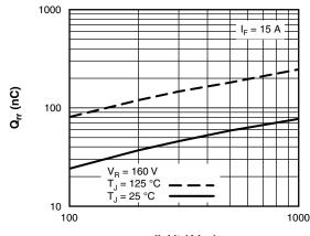
dl<sub>F</sub>/dt (A/μs) Fig. 10 - Typical Stored Charge vs. dl<sub>F</sub>/dt
