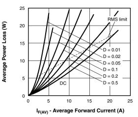
Fig. 8 - Forward Power Loss Characteristics
