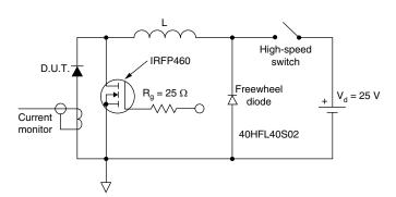
Fig. 8 - Unclamped Inductive Test Circuit
