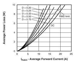
Fig. 6 - Forward Power Loss Characteristics
