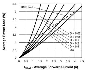
Fig. 6 - Forward Power Loss Characteristics
