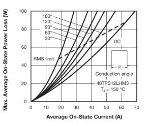
Fig. 4 - On-State Power Loss Characteristics
