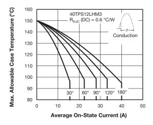
Fig. 1 - Current Rating Characteristics
