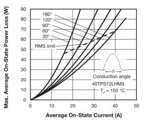
Fig. 3 - On-State Power Loss Characteristics
