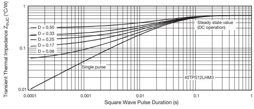
Fig. 9 - Thermal Impedance  $Z_{thJC}$  Characteristics
