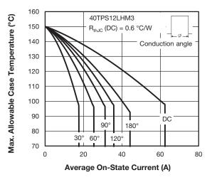
Fig. 2 - Current Rating Characteristics
