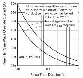
Number Of Equal Amplitude Half Cycle Current Pulses (N) Fig. 5 - Maximum Non-Repetitive Surge Current
