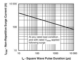
Fig. 7 - Maximum Non-Repetitive Surge Current (Per Leg)
