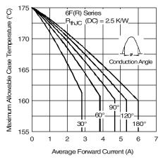
Fig. 1 - Current Ratings Characteristics
