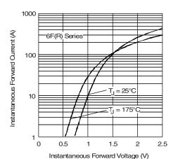
Fig. 7 - Forward Voltage Drop Characteristics
