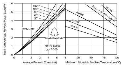
Fig. 3 - Forward Power Loss Characteristics
