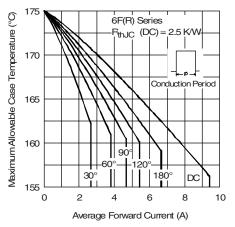
Fig. 2 - Current Ratings Characteristics
