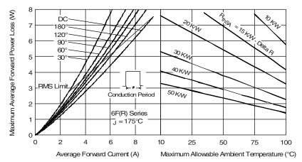
Fig. 4 - Forward Power Loss Characteristics
