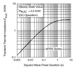
Fig. 8 - Thermal Impedance  $Z_{thJC}$  Characteristics
