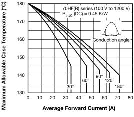
Fig. 1 - Current Ratings Characteristics
