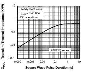
Fig. 12 - Thermal Impedance Z<sub>thJC</sub> Characteristics
