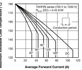
Fig. 2 - Current Ratings Characteristics
