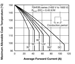
Fig. 4 - Current Ratings Characteristics
