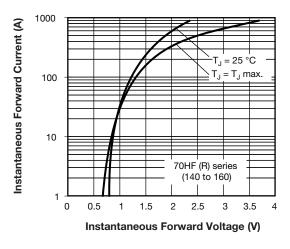
Fig. 13 - Forward Voltage Drop Characteristics
