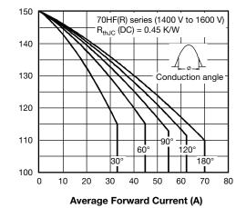
Fig. 3 - Current Ratings Characteristics
