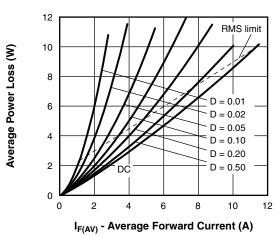
Fig. 6 - Forward Power Loss Characteristics
