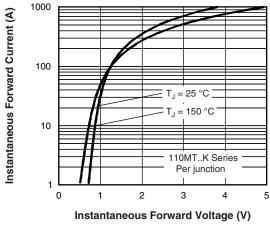
Fig. 7 - Forward Voltage Drop Characteristics
