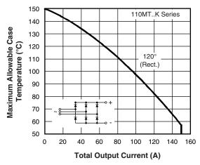
Fig. 6 - Current Ratings Characteristics
