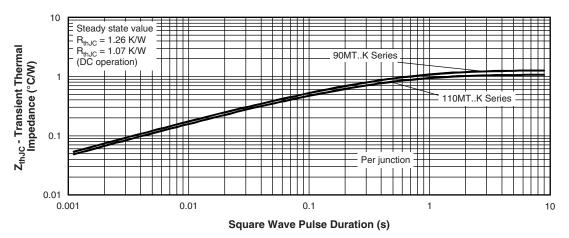
Fig. 11 - Thermal Impedance Z<sub>thJC</sub> Characteristic
