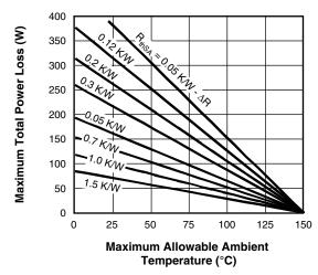
Fig. 3 - Total Power Loss Characteristics
