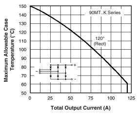
Fig. 1 - Current Ratings Characteristics
