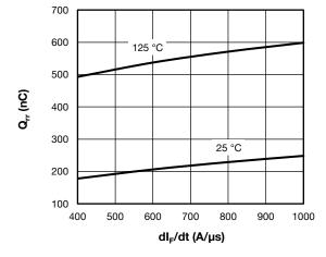
Fig. 8 - Typical Stored Charge vs. dl<sub>F</sub>/dt
