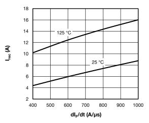
Fig. 9 - Typical Reverse Current vs. dl<sub>F</sub>/dt
