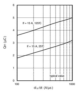
Fig. 8 - Typical Stored Charge vs. dl<sub>F</sub>/dt
