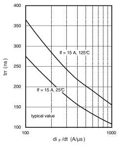
Fig. 7 - Typical Reverse Recovery vs. dl<sub>F</sub>/dt
