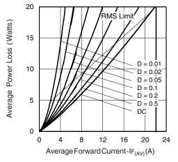
Fig. 6 - Forward Power Loss Characteristics
