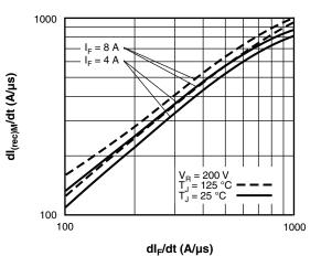
Fig. 8 - Typical dI<sub>(rec)M</sub>/dt vs. dI<sub>F</sub>/dt
