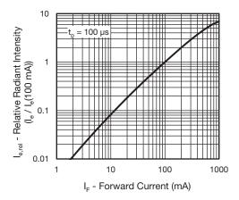
Fig. 4 - Relative Radiant Intensity vs. Forward Current
