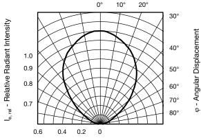
Fig. 9 - Relative Radiant Intensity vs. Angular Displacement
