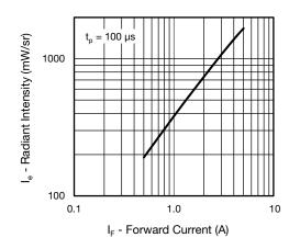
Fig. 6 - Radiant Intensity vs. Forward Current
