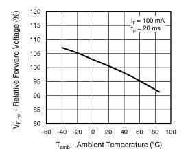
Fig. 5 - Relative Forward Voltage vs. Ambient Temperature
