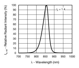
Fig. 8 - Relative Radiant Power vs. Wavelength
