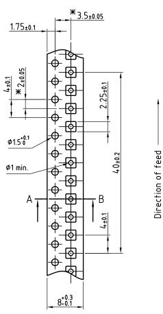
$^{f st}$  Measured from centerline of sprocket hole to centerline of pocket
