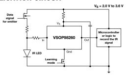
Recommended to minimize the connection distance between the IR LED and the input of the VSOP98260, and if possible to shield this connection to Gnd.
