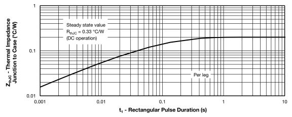
Fig. 8 - Thermal Impedance Z<sub>thJC</sub> Characteristics
