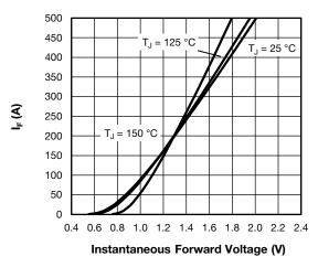
Fig. 7 - Typical Forward Voltage Characteristics
