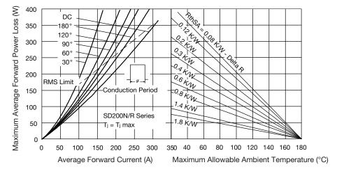
Fig. 4 - Forward Power Loss Characteristics
