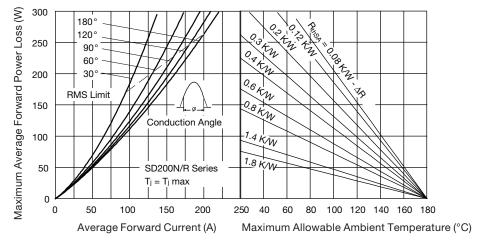
Fig. 3 - Forward Power Loss Characteristics
