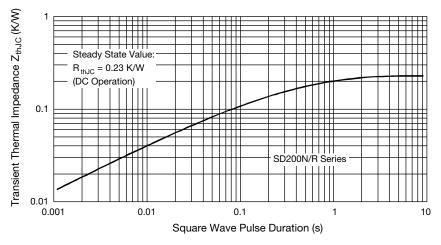
Fig. 8 - Thermal Impedance Z<sub>thJC</sub> Characteristic
