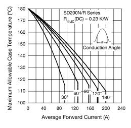
Fig. 1 - Current Ratings Characteristics
