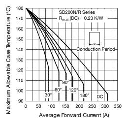
Fig. 2 - Current Ratings Characteristics
