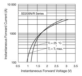
Fig. 7 - Forward Voltage Drop Characteristics
