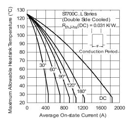
Fig. 4 - Current Ratings Characteristics
