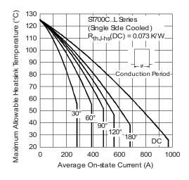
Fig. 2 - Current Ratings Characteristics
