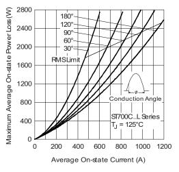
Fig. 5 - On-State Power Loss Characteristics
