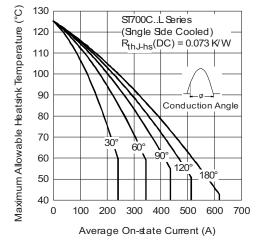
Fig. 1 - Current Ratings Characteristics
