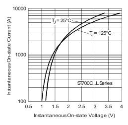
Fig. 9 - On-State Voltage Drop Characteristics
