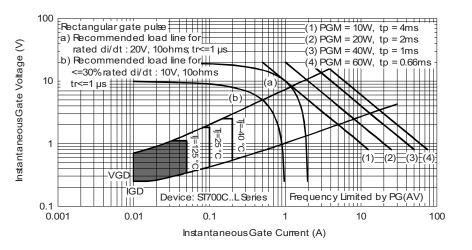
Fig. 11 - Gate Characteristics
