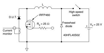
Fig. 8 - Unclamped Inductive Test Circuit
