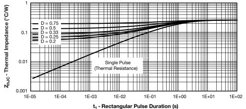
Fig. 4 - Maximum Thermal Impedance Z<sub>thJC</sub> Characteristics
