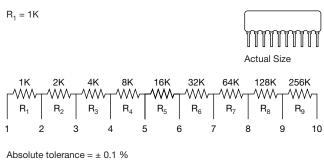
Absolute tolerance =  $\pm$  0.1 % Ratio tolerance =  $\pm$  0.1 % TCR tracking =  $\pm$  3 ppm/°C L = total length = 1.02" (25.91 mm) max. H = seated height = 0.280" (7.11 mm) max.
