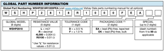
EB (lead (Pb) free) is a non-standard packaging code designated for 1000 piece reels. The non-standard packaging code is identical to our standard EA (lead (Pb) free), except that it has a package quantity of 1000 pieces
