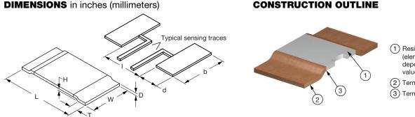
1 Resistive element: Fe-Cr (element material used is dependent on resistance value)
